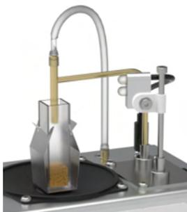
2. Put the cover assembly onto the Atomizer (1). Make sure that the four protruding tabs of the cover are fully inserted in the slots in the Atomizer shell. Move the latches to the close position (2) and tighten the locking screws (3).
